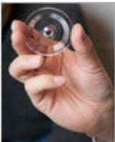
Until now, 3D microscopes required multiple lenses or multiple cameras to move around a tiny stationary object. At Ohio State University, researchers have introduced a proof of concept for the first stationary microscope lens that can produce true 3D images. This thermoplastic lens — designed using a computer program written by one of the researchers — [sees nine images at once](#).
